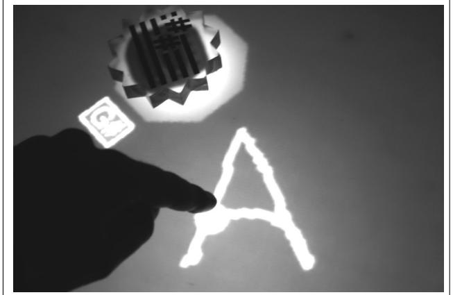
**Figure 5.** The action of drawing the letter A. Since there's no edit action associated with letter A, a new A major chord is going to be created.
